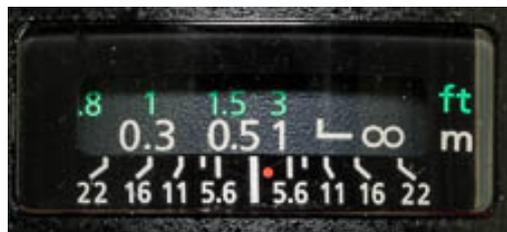
In the example above the 14mm lens is focused at the hyperfocal distance for f/11, which is 0.6m. With one f/11 mark aligned with the infinity mark ( $\infty$ ). The other f/11 mark is at 0.4m, which tells me that everything from 0.4m to infinite distance will be sharp if I use an aperture of f/11. This is the quickest and simplest way of focusing a prime wide angle lens for landscape and similar subjects.
